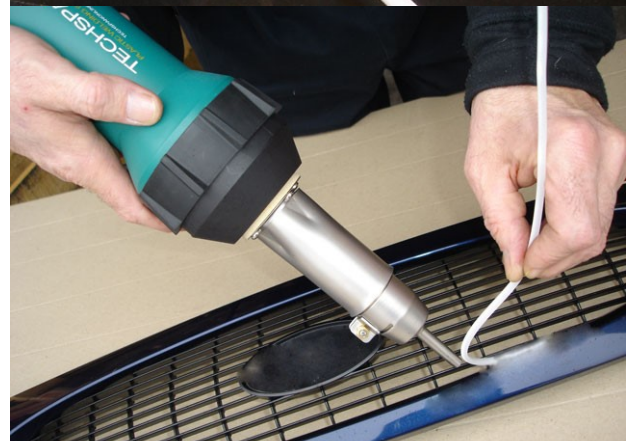
Pendulum Welding with standard nozzle
