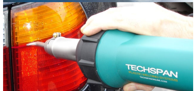
Tacking prior to welding
